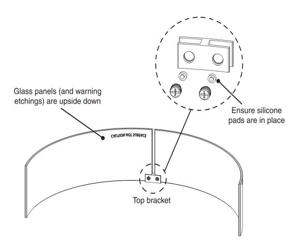
\*\*HINT: It is recommended to assemble wind guard upside down (as shown) for ease of assembly and flip over after it is fully assembled.\*\*
